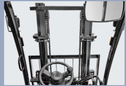
Ultra-wide-view mast and the front view of the driver broadened by 8%
